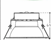
Ceiling Cut-Out: 6-3/4" Ø
