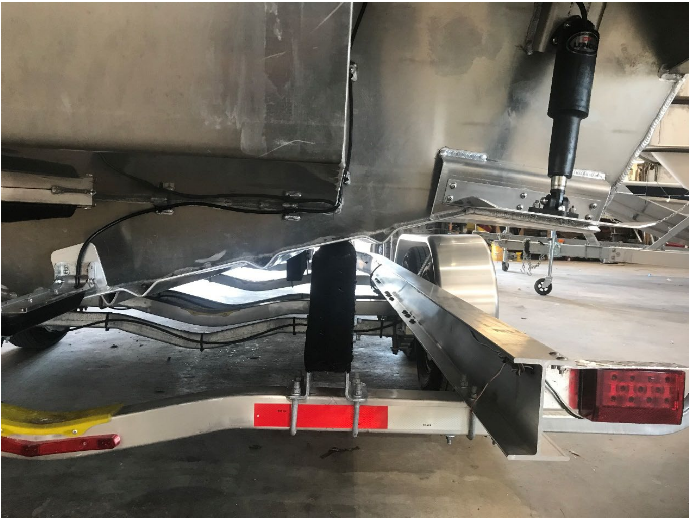
Photo #1: Reverse Chine Stabilizers 5.5°
