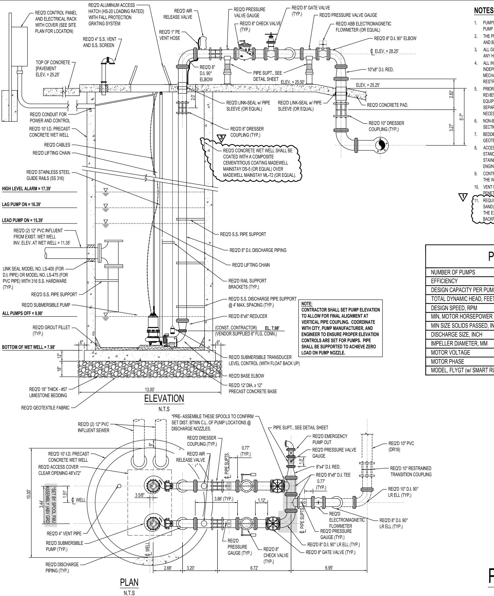
1. PUMPS, GUIDE RAILS, BASE ELBOWS, AND ACCESS HATCHES SHALL BE SUPPLIED BY THE PUMP SUPPLIER, OR CERTIFIED AS COMPATIBLE BY THE RESPECTIVE MANUFACTURERS. 2. THE PRECISE LOCATION OF HATCHES, AND LOCATION/ SPACING OF PUMPS, GUIDE RAILS, AND BASE ELBOWS, SHALL BE AS RECOMMENDED BY THE MANUFACTURER.
