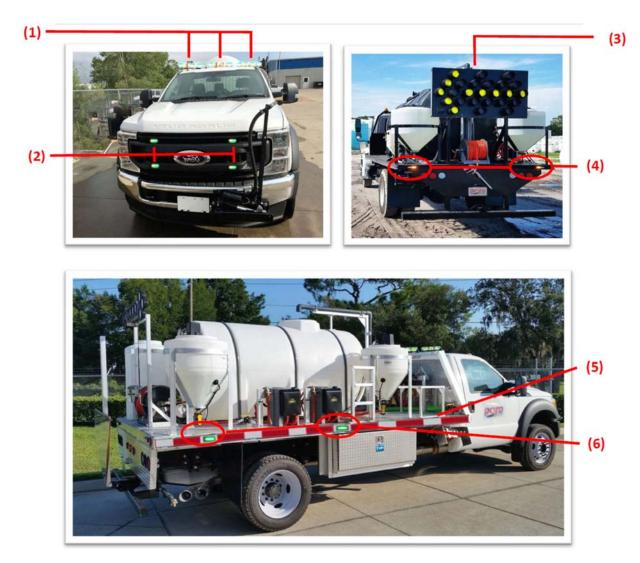
Note: This image represents the locations for safety lighting on the truck (Arrow board shown in the image above labeled as #3 is not required)
